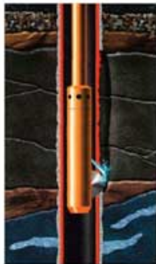
Hydro- Sandblast Jet-assisted mechanical slot perforation
